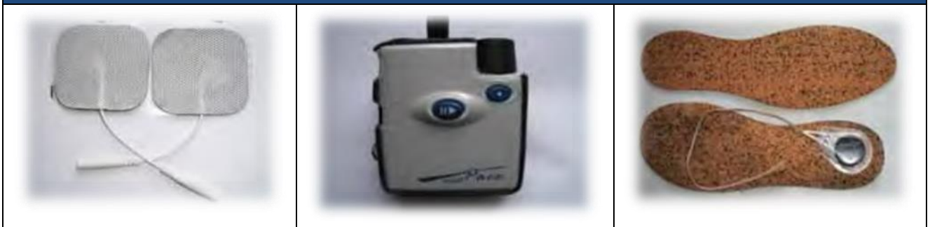
Above: left – sticky pads for your legs, centre: control unit for your belt , right insoles with heel strike pad for your shoes
